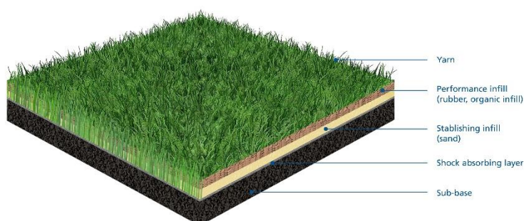
Figure 1: composition of a third-generation football turf system ©FIFA
