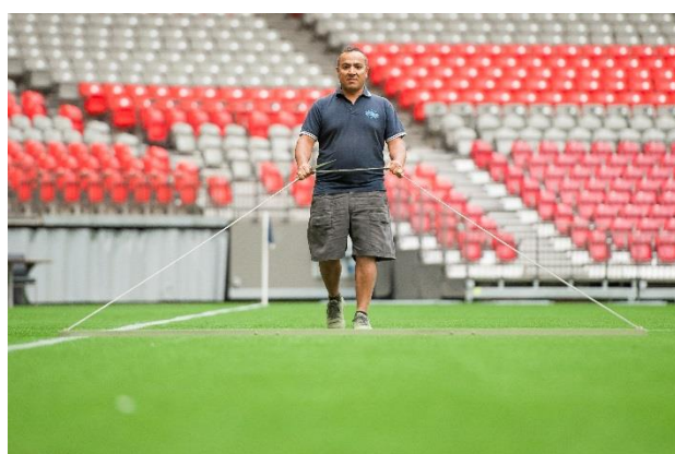
Figures 4 & 5: ball roll and straight edge test by a FIFA-accredited test institute prior to the FIFA Women's World Cup Canada 2015™ ©Getty Images
