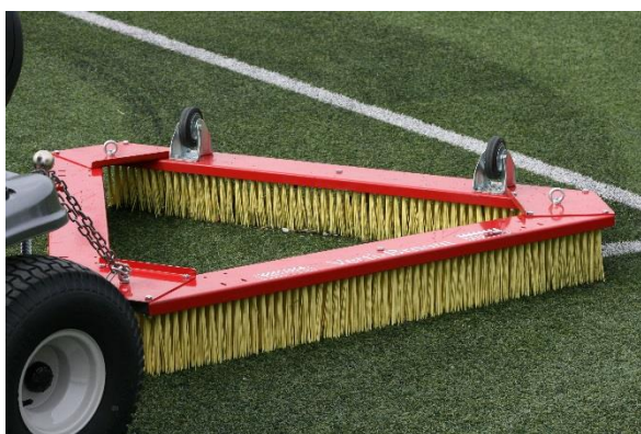
Figure 11: triangle brush attached to a tractor for basic brush action ©FIFA
