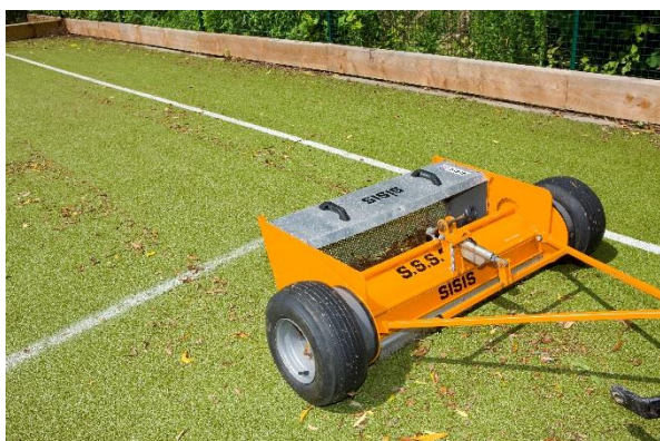
Figure 14: rotating brush to remove debris from the surface ©Sisis
